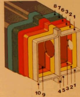
But Peugeot does not stop there. Eight other processes, before and after the electrophoretic bath, add up to 50 lbs of well-established anti-corrosion coatings of proven resistance value.
